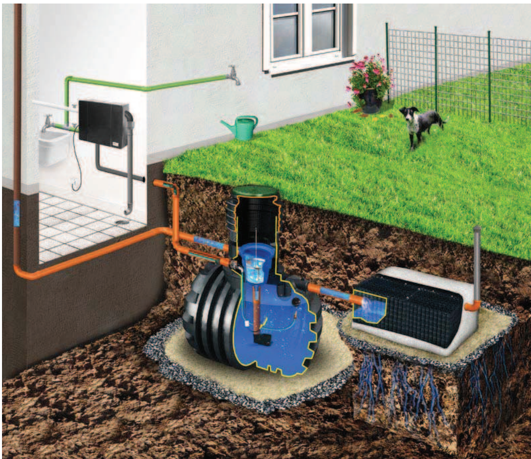
House Complex I - system with collecting filter
